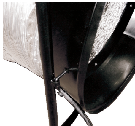
FIG 2 – Detaching of the connecting flange
